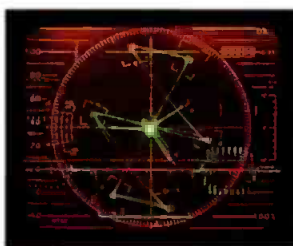
Combination Display— Simultaneous waveform and vector displays of a single input
